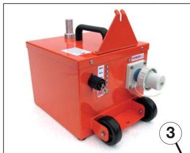
Battery case with built-in intelligent analyser/charger, 110/230 volt AC socket, 12 volt DC outlet, carrying handle and folding base legs, containing a 12 volt 40 Ah maintenance-free rechargeable battery.
