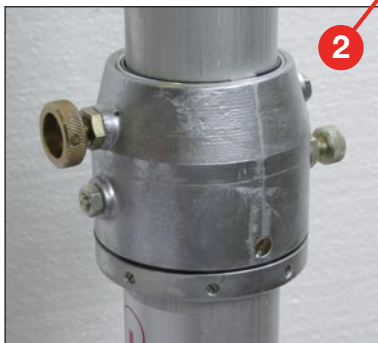
Lockable rotating collar, standard natural clear anodised seamless drawn aluminium mast sections with Ø 2½" (63,5 mm) base tube
